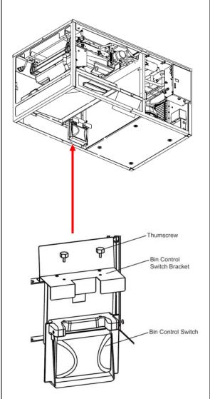
The IM-500SAA uses a mechanical bin control located on the right rear side of the ice drop zone. This control will open when ice pushes against the switch, if the switch stays open for more than 10 seconds the machine will start the bin control cycle, starts and the machine will shut down after the next defrost cycle.
